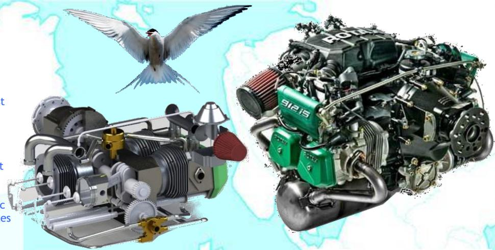
912iS CAD model above, and Rotax 912iS benchmark off-the-shelf engine above right. [PDF](#)
